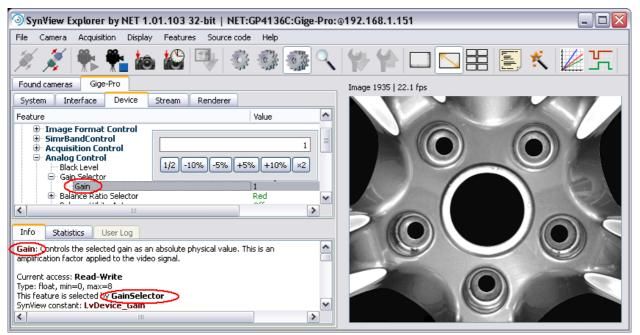
Figure 9: SynView Explorer: Setting gain — note about the Gain selector
